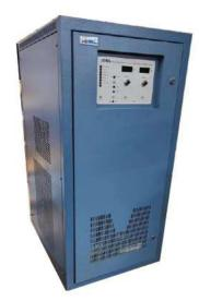
High Power Series range regulated and variable DC power supplies are solid state units utilizing thyristor technology in a single and three phase full-bridge rectifier topology that offer constant voltage control, constant current control, automatic crossover, series regulation, DC filter, digital metering and various operational and protective monitoring features.
