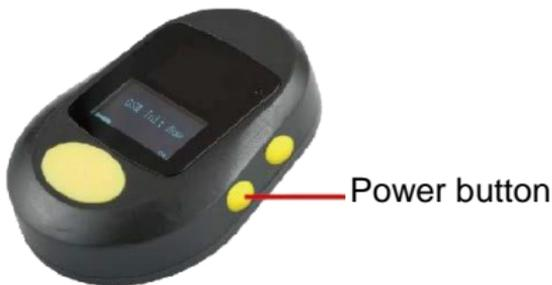
**Note:** For the first time turning ON the device, please put the device outside so it can upload all the settings and your local GPS coordinates.
