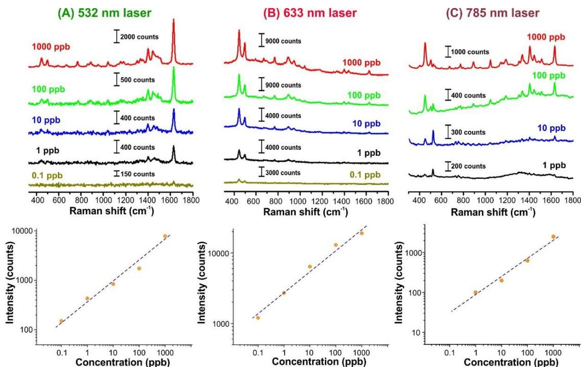
**Figure 2.** (A – C) SERS spectra of methylene blue (MB) at various concentrations measured using 532, 633 and 785 nm excitation laser wavelengths, respectively. *PowerSERS* substrate allows the detection of MB probe molecule down to part-per-billion levels (0.1 – 1 ppb detection limit) using different laser wavelengths.
