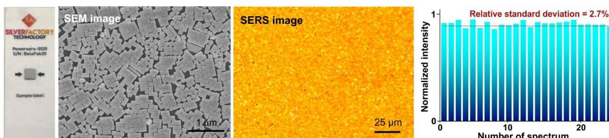
**Figure 1.** A digital photograph, SEM image and SERS image of PowerSERS. The SERS signal variation is <3% across a large area.
