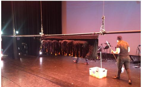
Photo above of the flower petal dropping device. The device is made of fabric and two pieces of wood that run laterally. The fabric has deep slits that hold the petals in place. The petals are released when a stage manager lightly shakes/moves the pipe that the device is mounted on. The device cannot be on the same pipe as hanging scenery, but is ideally located as close to the mid traveler as possible, preferably downstage of the hanged scenery.
