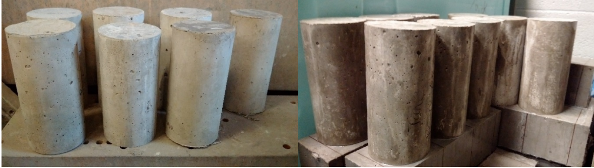
Figure 2: Cylinder specimens in the conditioning room: a) Dry curing, b) Moist curing
