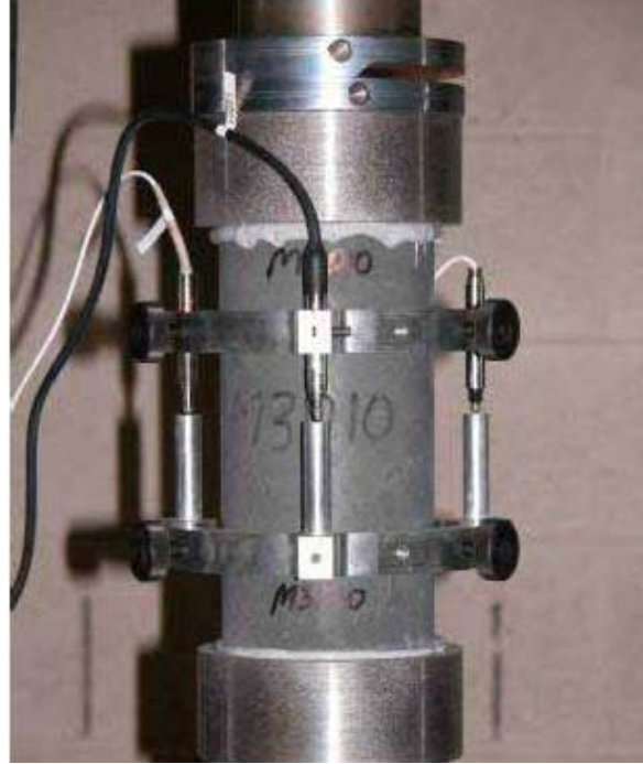
Figure 3: Test set up for determining cylinder compression strength
