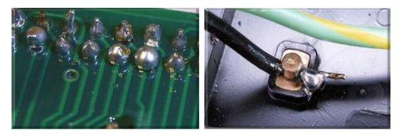
**(Left)** A tenfold excess of solder on this hand---soldered printed circuit board, and (extreme left) an incomplete solder joint with poor coverage. There is no need to add more solder "for luck".
