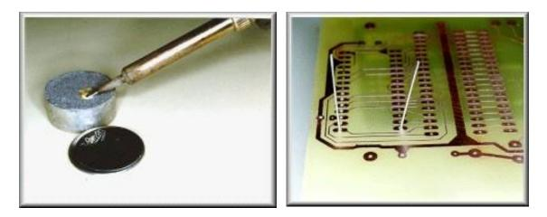
(Left) A useful product is Multicore's Tip Tinner Cleaner (TTC) - a 15 gramme tin of special paste which cleans and "tins" the soldering iron iron, in one go. New tips must be tinned **immediately** when used for the first time. (**Right**) Insert components and splay the leads so that the part is held in place.
