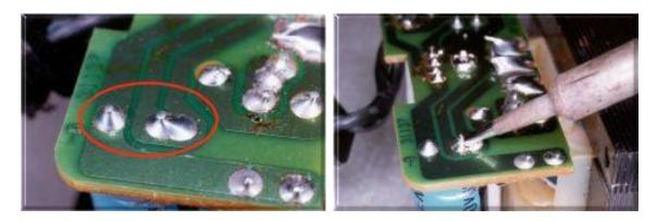
**(Left)** The two solder joints to be desoldered, to enable a faulty electrolytic capacitor to be removed from the printed circuit board.
