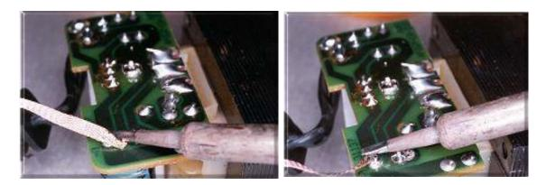
(Left) Select a suitable width of desoldering braid, and **press it down** onto the COLD joint using the hot tip of the iron. A flat soldering iron bit is preferable.
