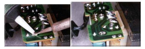
**(Left)** The PTFE nozzle of the desoldering pump is applied to the molten solder and the spring---loaded plunger is then immediately released, drawing the molten solder up into the pump. Remove the soldering iron tip. Repeat the process if needed. *Handy tip*: sometimes it helps to add some fresh solder and then desolder the whole joint.
