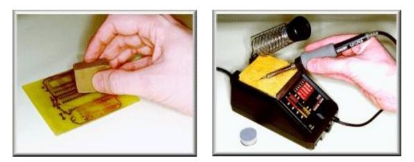
(Left) Printed circuit board copper tracks must be clean to begin with, especially if they're not previously "tinned" with solder. Clean any raw p.c.b. copper tracks gently with e.g. an abrasive rubber block available from electronics suppliers. (**Right**) Clean the iron "bit" (soldering iron tip) using a damp sponge. The soldering iron featured is an Ungar Concept 2100 Soldering Station. Other popular brands of soldering equipment include <u>Weller</u> and <u>Antex</u>.
