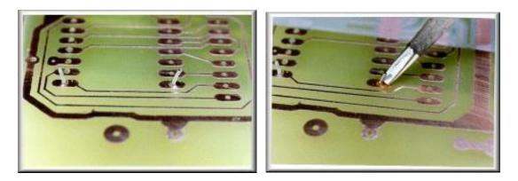
(Left) It's usually best to snip the electronic component wires to length prior to soldering. This helps prevent transmitting mechanical shocks to the copper foil.(**Right**) Apply a clean soldering iron tip to the copper solder pad and the component lead, in order to heat *both* items at the same time.
