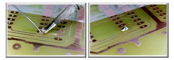
(Left) Continue heating and apply a few millimetres of solder. Remove the iron and allow the solder joint to cool naturally. (**Right**) It only takes a second or two, to make the perfect joint, which should be nice and shiny. Check the Guide for troubleshooting help.
