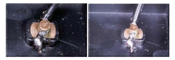
**(Left)** How **not** to make a mains voltage soldered joint. This solder joint went "dry" and starting arcing, nearly destroying the attached equipment. It is also a fire hazard.
