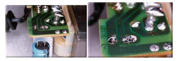
**(Left)** The faulty electrolytic capacitor dropped out of the board after desoldering. Sometimes, it may need persuading with pliers.... but don't overdo this or you risk damaging the copper tracks on the p.c.b.
