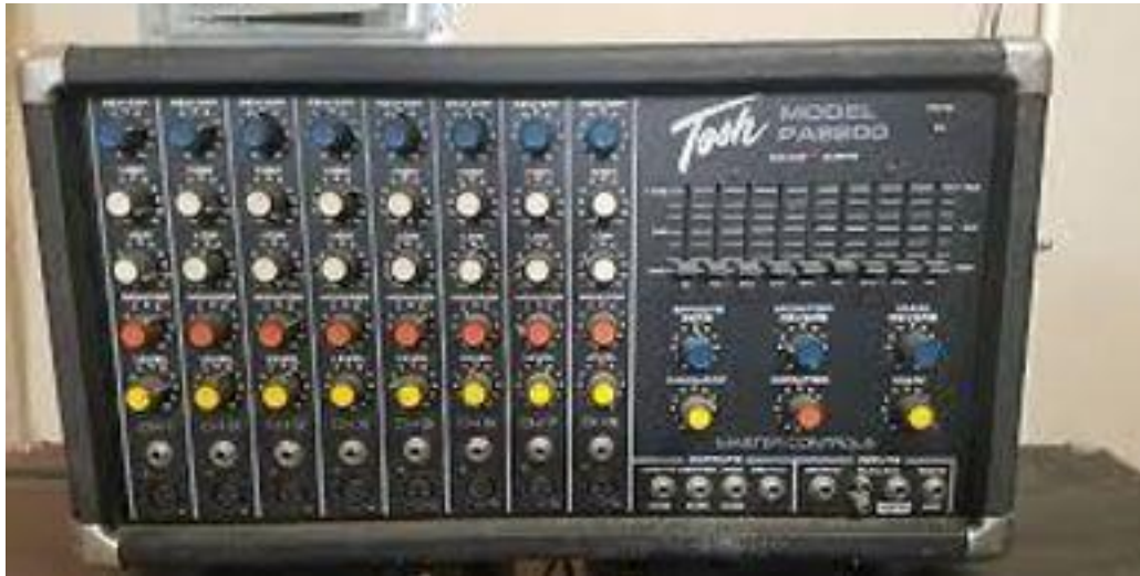
Tosh PA8250-P 8 Channel P.A. System: 250 Watts @ 4 Ohms, hi and lo impedance inputs, built in accutronics reverb, 9 band graphic equalizer, effects loop
