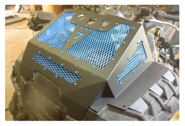
Mark and Drill 4 holes along sides. Front holes do not need drilled.
