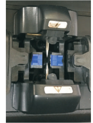
12. Close the electrode cap, electrode replacement is complete
