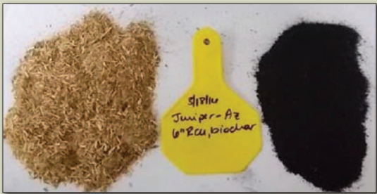
Juniper biomass converted to biochar. Photo Credit: Upper Verde River Watershed Protection Coalition (UVRWPC)
