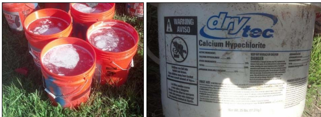
Figure 3-5 Buckets of super-chlorinated water (left) and calcium hypochlorite (right)
