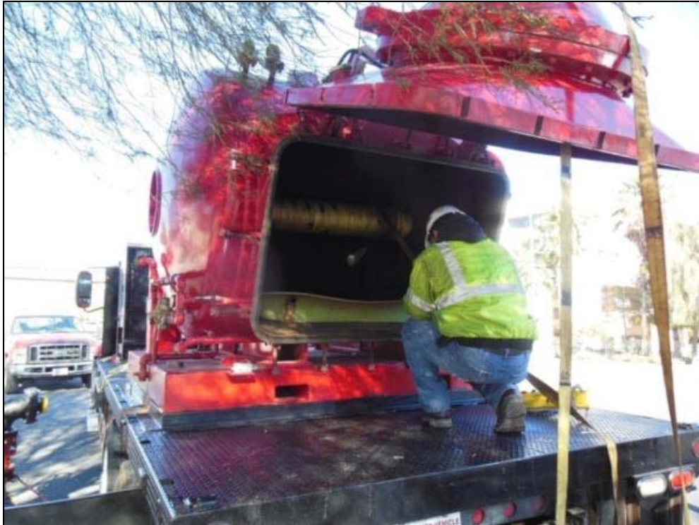
Figure 4-6 Pressure vessel mounted on the inversion truck
