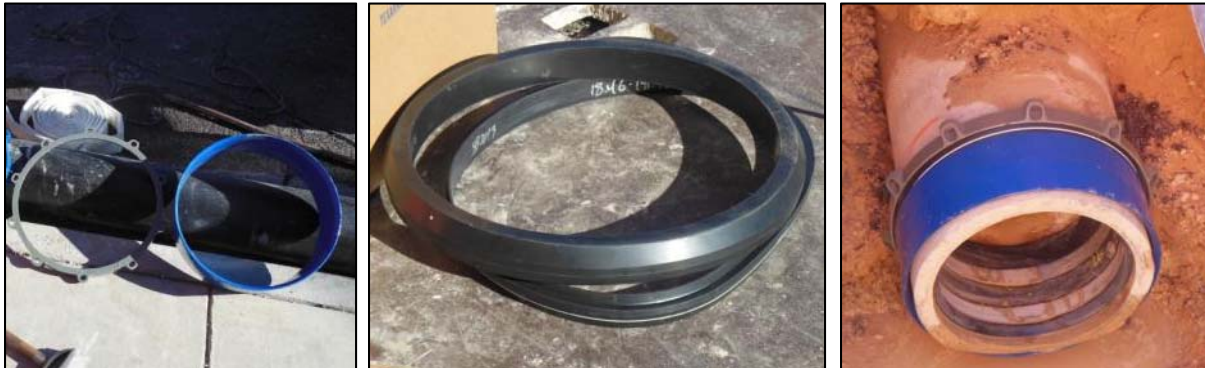
Figure 4-20 Sleeve and flange (left); rubber gasket (center); connection fitting (right)
