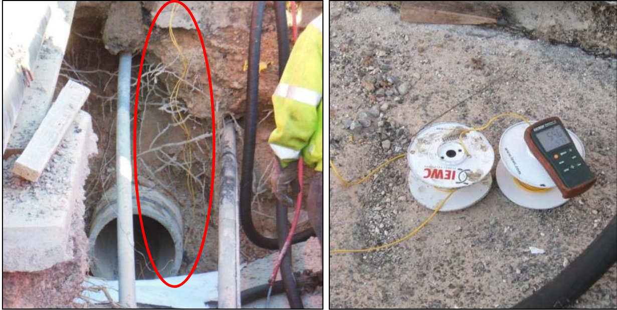
Figure 4-14 Yellow thermocouple wire inside pipe (left) and digital thermometer (right)
