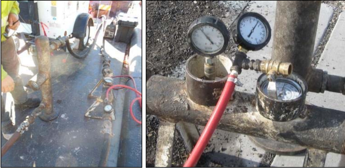
Figure 4-12 Pressure and temperature apparatuses with gauges
