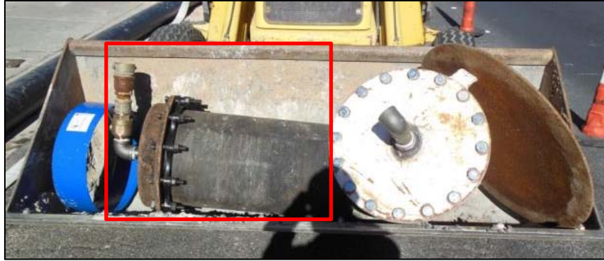
Figure 4-19 End cap assembly used for pressure testing
