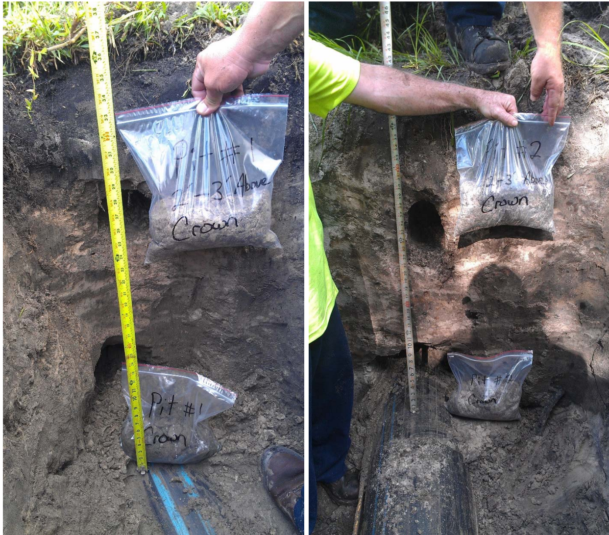
Figure 3-21 Retrospective soil samples from AC pipe bursting site
