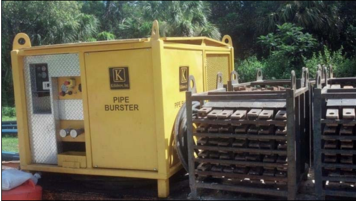
Figure 3-10 Hydraulic pump and linkages on a trailer
