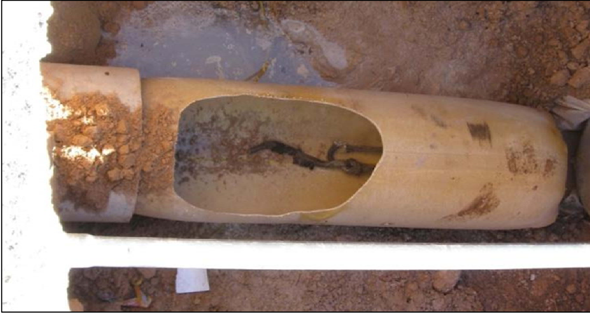
Figure 4-16 Cured liner with section removed to gain internal access to black rope
