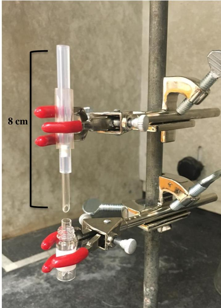
Figure 2.2. VOCs were eluted from the Hayesep® Q into 1.5 ml SureStop™ GC vials containing a 9.0 mm 300  $\mu$ l insert with 150  $\mu$ l of dichloromethane (Sigma-Aldrich, St. Louis, MO, USA) injected into the trap which was pushed gently through with  $N_2$ . An additional 5.0  $\mu$ l of n-Octane at a concentration of 80 ng/ $\mu$ l was added to each sample as an internal standard.
