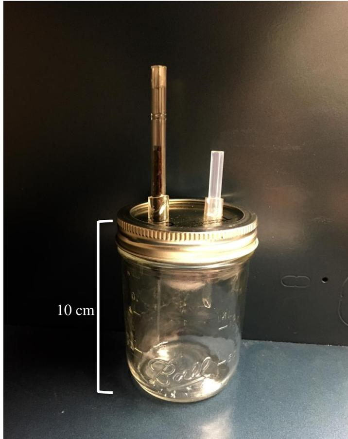
Figure 2.1. Headspace collection set up used to collect volatiles from manure samples. A 236.5 ml Ball® mason jar was outfitted with two holes in the lid: one for a carbon filter to purify ambient air (left) and another for the volatile trap (right). Volatile traps contain 30.0 mg of porous polymer mix Hayesep® Q to which volatiles adhere to. Samples of 20g were placed at the bottom while air was pulled at 1.0 L per min for 1 hr.
