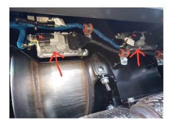
**Step 2** Locate nox sensors and make sure you have two a inlet and outlet nox labeled B5502 and B5503
