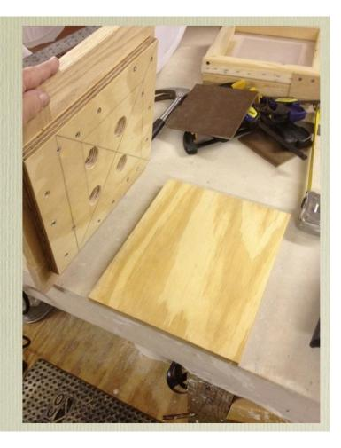
Lay the completed press exactly on top of the other 10 x 12-inch sheet of plywood.
