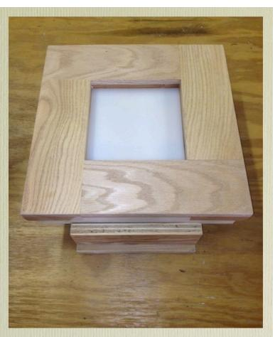
The press on top of the punch. Push it away from you and the tilemaker drops onto the punch dowels.
