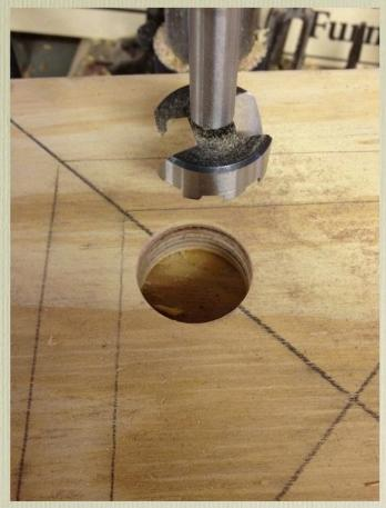
A "Forstner" bit in a drill press will make a neat hole, but you can use a hand-held drill as well. Neatness will not affect function.
