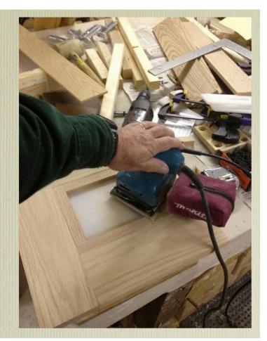
Sand the surface with a power sander or a flat block of wood with sandpaper on it.
