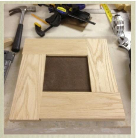
Place the 6-inch Masonite® square into the tilemaker to check the fit.
