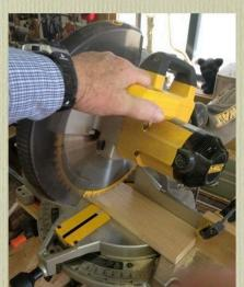
Cut four half-inch-thick by four-inch wide hardwood boards to 10-inch lengths. These form the top surface of the tilemaker. Place the first board just inside the line you drew previously.
