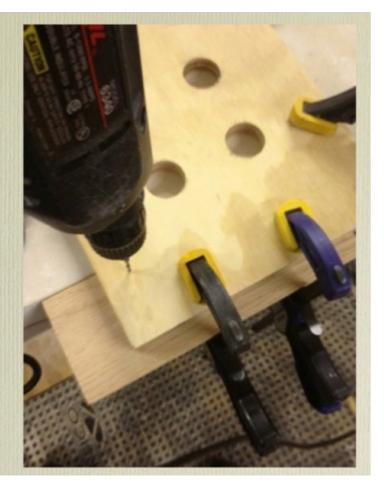
From the backside, pre-drill screw holes through the plywood into the hardwood board while it is clamped in place.
