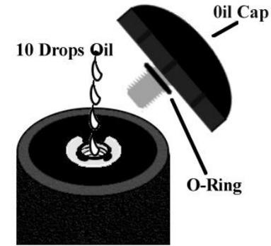
2. Fill the oil reservoir with cutting wheel oil (available at your local stained glass distributor).
