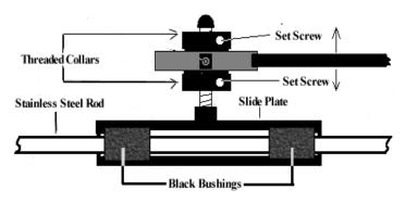
Loosen the screws in the threaded shaft collars. Turn the threaded collars to adjust the arm up or down the desired amount. Re-tighten the screws, being careful not to over tighten.
