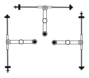
NOTE: Having the spring closer to you allows you to easily set up Cutter's Mate on a Morton grid. If you decide to use The Waffle Grid, you will need to use the grid adapters so that Cutter's Mate will maintain a constant 90-degree angle when scoring glass.
