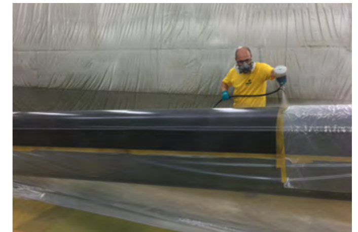
The surface coated with Berucoat AF 339 for telescoping is dry to the touch after one hour, can be subjected to load after 3 days, and after 7 days it has cured.
