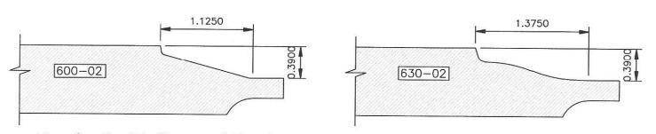
Most of our Panel Profiles are available with an "-02" option. The option adds additional thickness to the back of the panel. Two examples of this are shown above but we did not draw out the option for every available Panel Profile.
