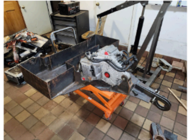
Tesla rear drive unit on a custom-built subframe that integrates the motor mount and rear battery box into a single unit.
