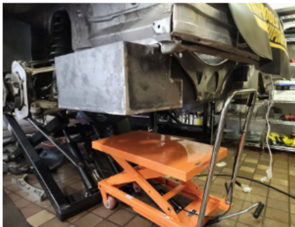
The subframe houses one of the two 48S2P battery packs (6 modules).
