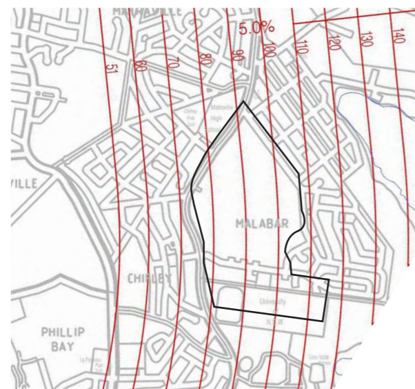
Obstacle Limitation Surface constraints on the site
