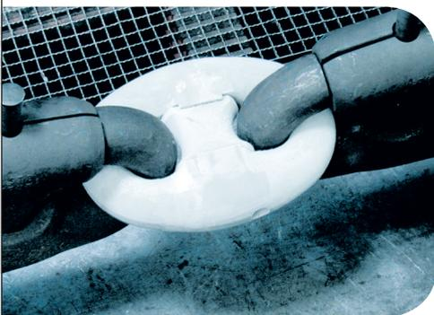
**The parts have been MBL tested up to -40° C**
