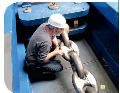
**High cycle fatigue tests have been witnessed by DNV.**
