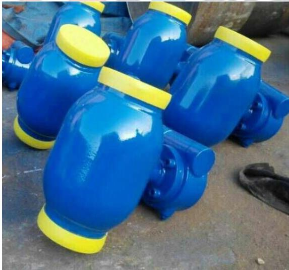
Fully Welded ball valve
