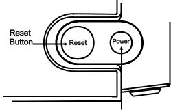
Power Off/On Button There are two styles of top panels. Illustrated here are the two different styles.
