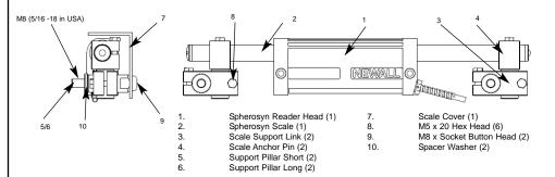
Figure 2 - Microsyn Encoder Assembly
