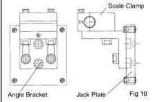
Mount the reader head as before, ensuring that the rounded edge is facing downwards.
