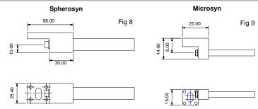
For Spherosyn remove cheese head nylon screw from end of scale. Do not tamper with the adjustment set screw as this will alter the calibration.
