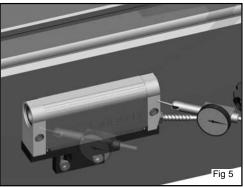
The reader heads should be mounted with both planes parallel to the axis of travel within +/- 0.05mm(0.002"). See fig 4 and 5.
