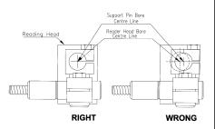
Traverse the machine to its maximum position towards the non cable entry side of the reader head. Slide scale through reader head and fit assembly (fig 6 & 7) onto end of scale. Mark the position of the nillar
