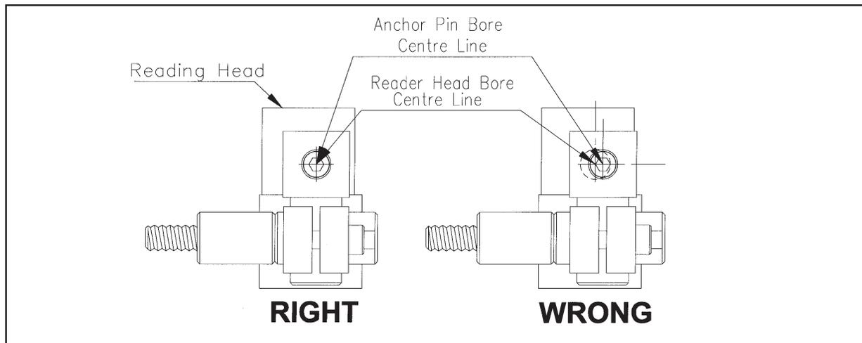
**Figure 5.9 - Reader Head and Bracket Alignment**
