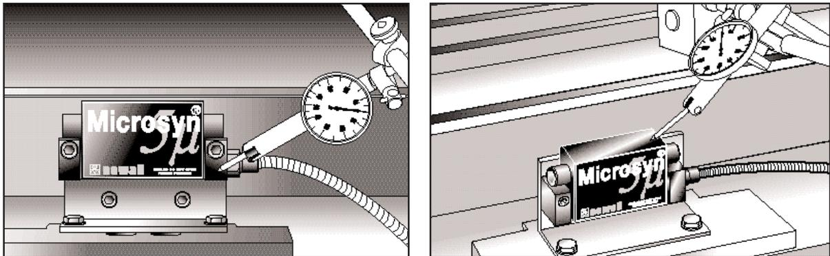
*Figure 4.2 - Alignment of the Microsyn Reader Head*
