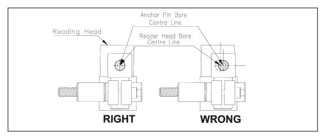
Figure 5.9 - Reader Head and Bracket Alignment
