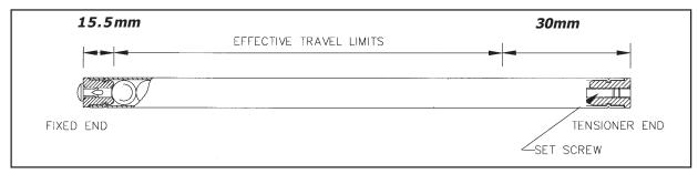
Figure 5.1 - Spherosyn Scale
