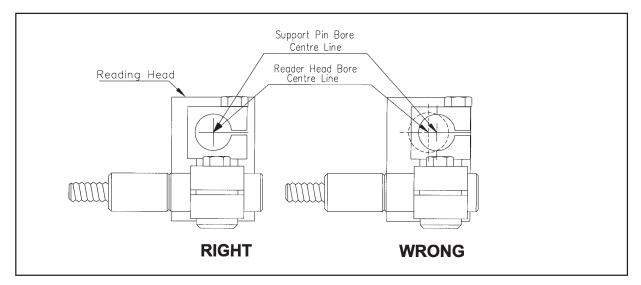
Figure 5.2 - Reader Head and Bracket Alignment
