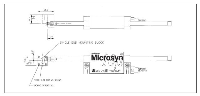
Figure 5.10 - Microsyn Single End Mounting
