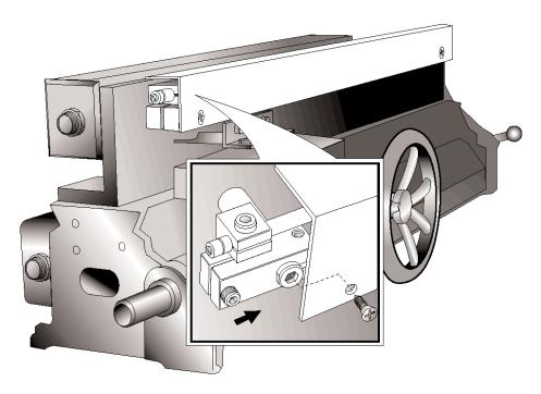
Figure 6.1 - Fitting the Scale Guard (example shown using a Spherosyn Scale)
