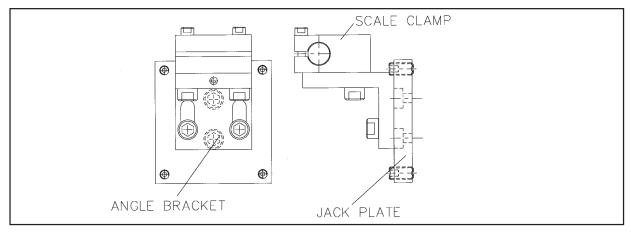
Figure 5.5 - Long Scale Support Bracket Assembly
