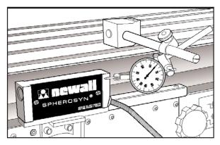
Figure 4.1 - Alignment of the Spherosyn Reader Head
