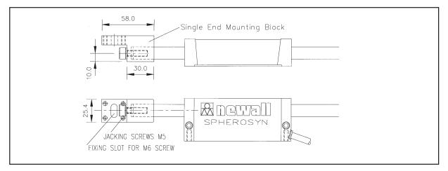
Figure 5.4 - Spherosyn Single End Mounting
