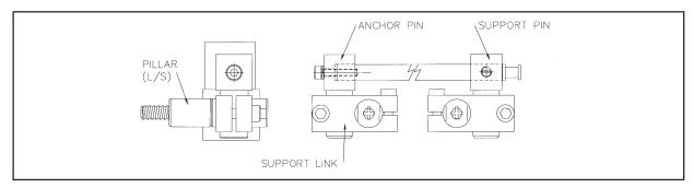
Figure 5.8 - Microsyn Scale Support Bracket
