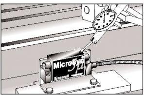
Figure 4.2 - Alignment of the Microsyn Reader Head
