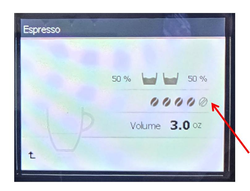
When pouring a drink, you can use the rotary switch to adjust the strength of the drink. This option disappears fast, so have your hand on the rotary after choosing an option. The coffee beans will show the strength.
