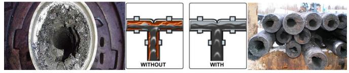
Paraffin removal from the inside of your tubing on plunger lift, rod pumped and flowing producers presents a problem for many oil and gas producing wells. Our proprietary process
