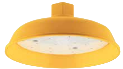
Model 01054005 Shower Head Assembly, Yellow ABS, integral 20 gpm / 113.6 lpm regulator, 1" / 2.5 cm connection
