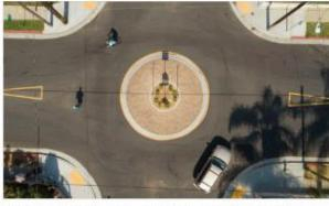
A **traffic circle** is a raised island located in the center of an intersection around which traffic must circulate. They may be used to lower vehicle speeds and conflicts at the intersection of two roadways. They are typically operated as two-way or all-way stop-controlled intersections
