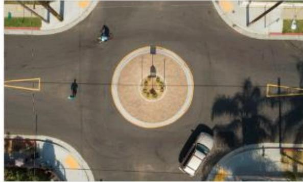
A **traffic circle** is a raised island located in the center of an intersection around which traffic must circulate. They may be used to lower vehicle speeds and conflicts at the intersection of two roadways. They are typically operated as two-way or all-way stop-controlled intersections.
