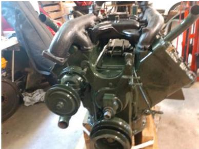
Freshly overhauled Cadillac/Lasalle engine 346 CID. New pistons, rings, oil pump, valves honed, crank ground. Has been test run.
