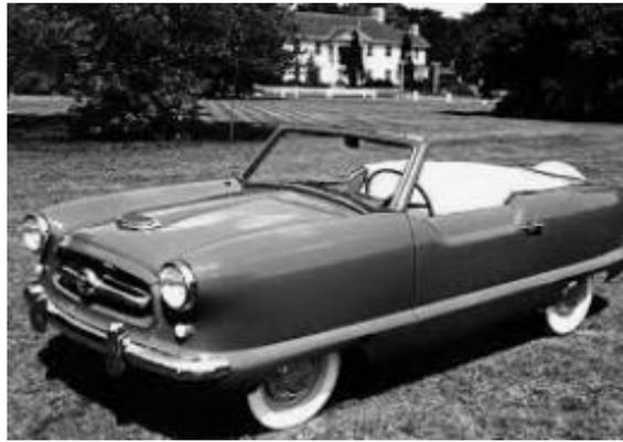
In August 1954 the Series II began. It now had the Austin B type 1200cc low compression engine, with a new redesigned block, water pump, fuel pump and head. The 7 ¼ inch clutch remained. Sunburst Yellow and Coral Red colors were added. The hood scoop and the 'propeller' type grill were carried over from the Series I along with the single tone paint scheme.
