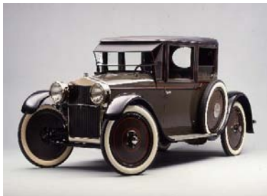
Brown designed the aluminum body; Fleetwood built and finished it in 1925.
