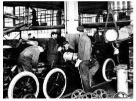
Mr. Ford is properly credited with the first known moving assembly line; this 1913 advance was a huge improvement. It was so good that it allowed Ford to build cars inexpensively, quickly, and to be affordable. The Model T Ford was massively successful. This was due to an excellent design that efficiently used standardized parts. In addition, Model Ts were reliable, economical, easy to operate, maintain, and repair.
