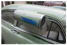
In hot, dry climates, another non-power, very nice option back then was water-filled evaporative coolers. These cylinder-shaped devices were placed outside of the car, attached to the door frame, and had an air vent that entered the mostly rolled up window. They were situated so that ambient air would pass into the cylinder's frontal opening while the car was moving, blow outside air over wet fiber in the water-filled container, and then vent cooler, damp air into the passenger compartment. My
