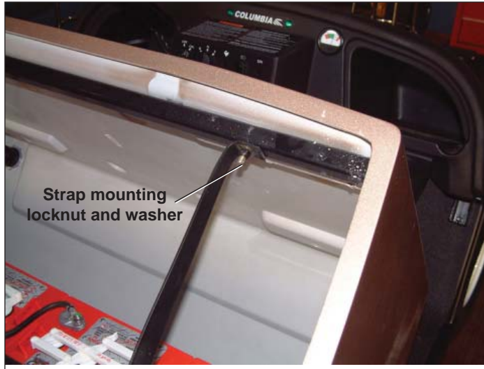
Figure 8-9. Middle Body Strap Mounting
