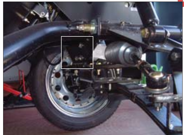
Figure 6-6. Rack & Pinion to Frame Mounting
