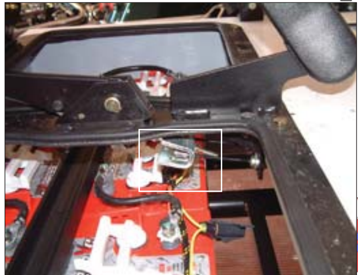
Figure 5-12. Parking Brake Adjustment
