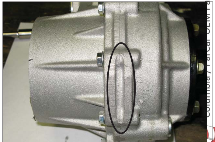
Figure 6-63. Pry Points at Bottom
