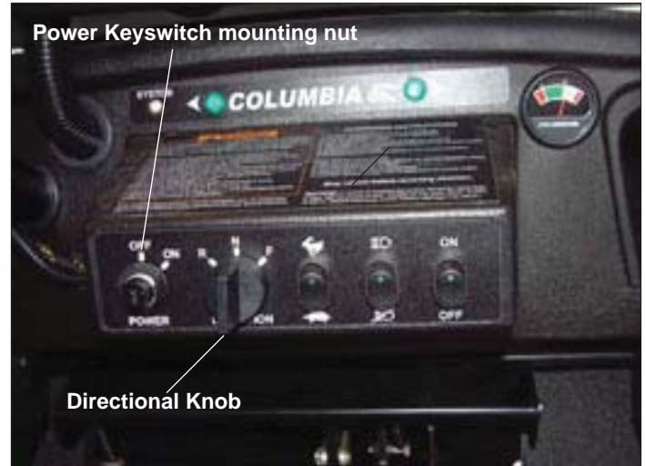
Figure 7-6. Power Keyswitch Mounting Nut (Console)
