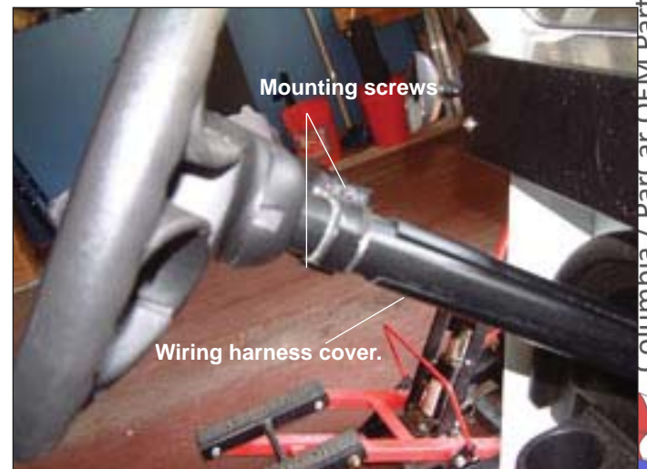
Figure 7-7. Turn Signal Assembly Mounting
