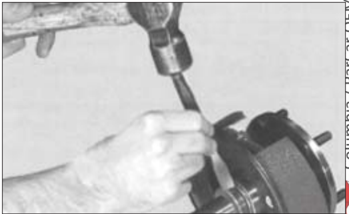
Figure 6-28. Removing Retaining Ring
