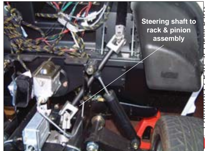
Figure 6-5. Rack & Pinion to Steering Shaft
