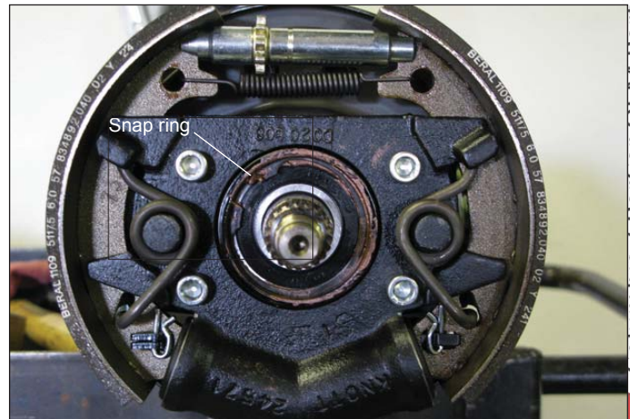
Figure 6-59. Removing Snap Ring
