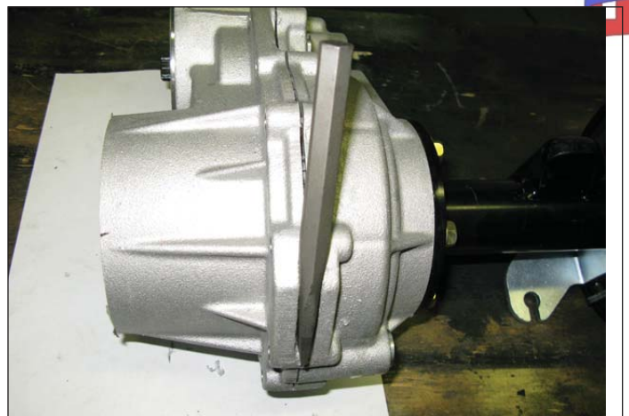
Figure 6-64. Pry Points at Top
