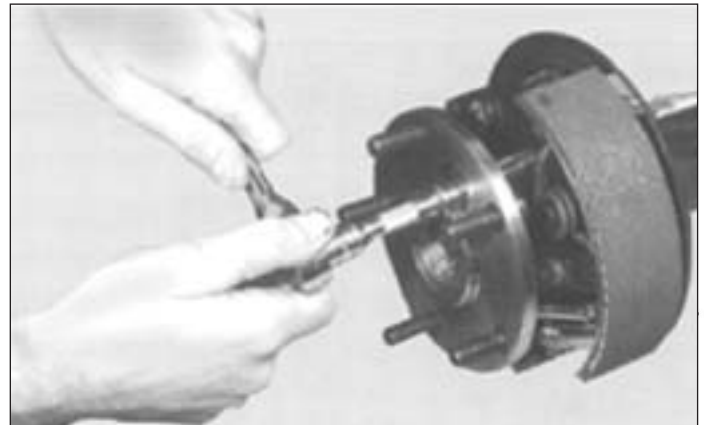
Figure 6-23. Removing Backing Plate Nuts
