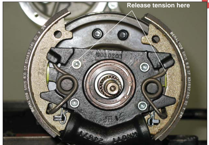
Figure 5-8. Rear Drum Brake - TEAM Axle Models
