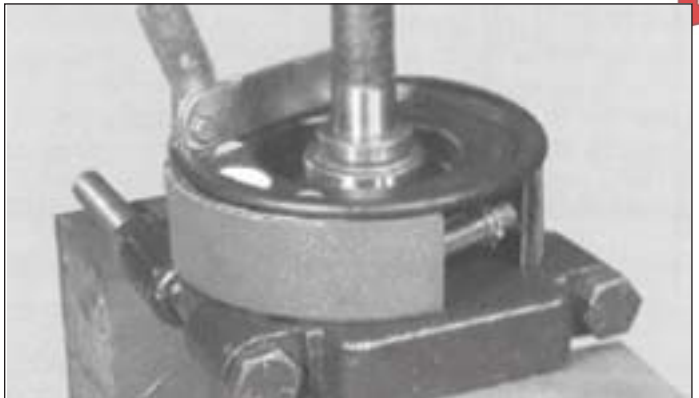
Figure 6-29. Removing Wheel Bearing and Brake Assy
