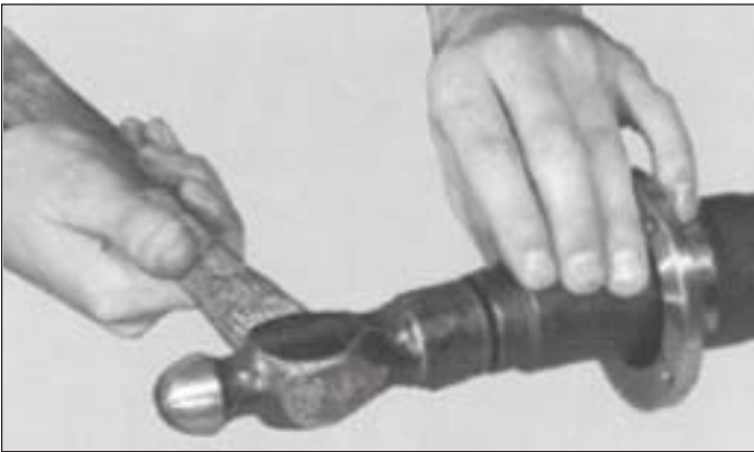
Figure 6-35. Assembling Grease Seal
