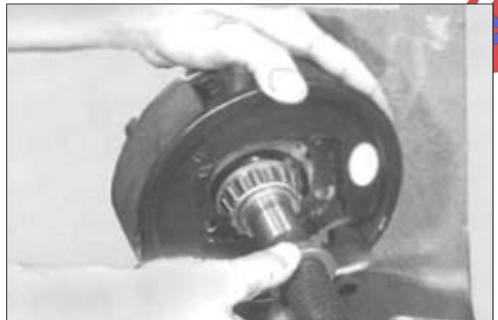
Figure 6-33. Retaining Ring on Axle Shaft
