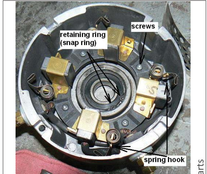
Figure 9-16. Spring Hooks for Brush Springs
