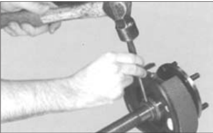
Figure 6-26. Removing Center Punch Retaining Ring
