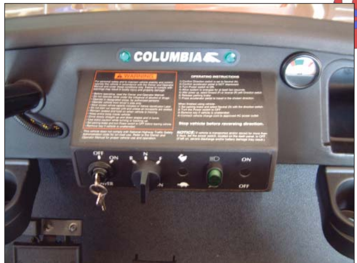
Figure 1-1. Warning and Operating Instructions Decal on Console
