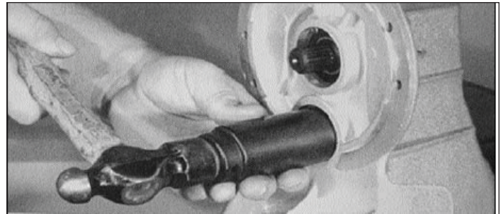
Figure 6-54. Installing Cup Plugs
