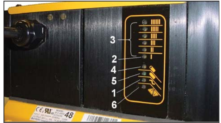
Figure 8-4. Delta-Q Charger and Lights
