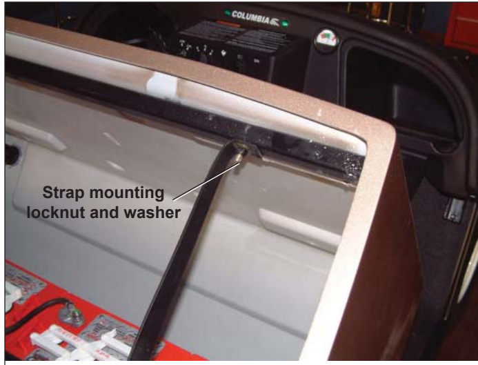
Figure 8-9. Middle Body Strap Mounting
