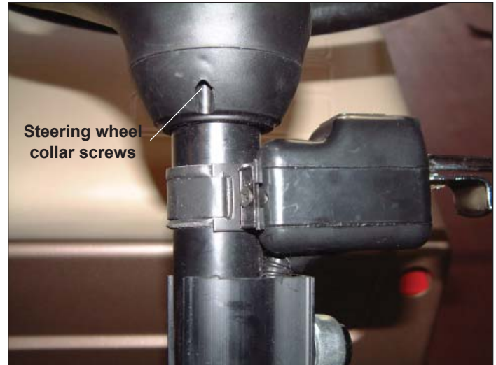
Figure 6-6. Steering Wheel Collar Mounting
