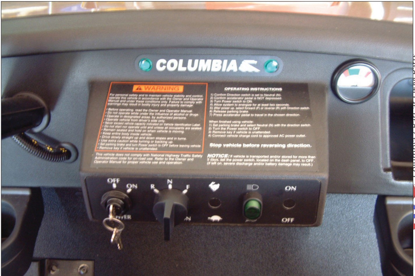
Figure 1-1. Warning and Operating Instructions Decal on Console
