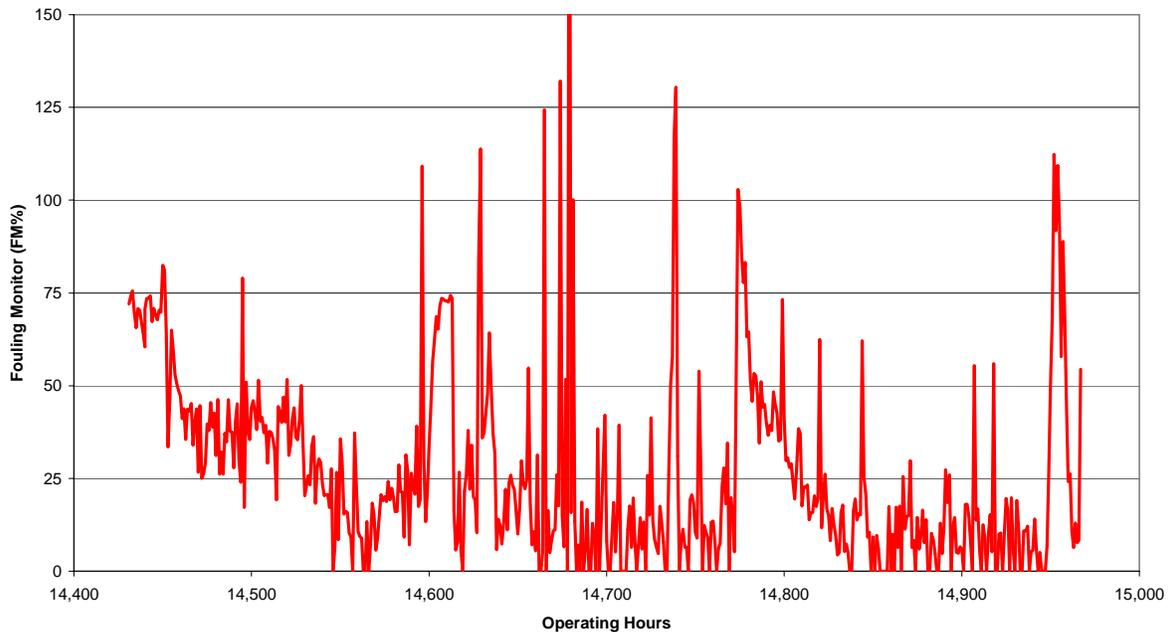
**Figure 7. MASAR® Foulings Monitor during the acid dosing trial**
