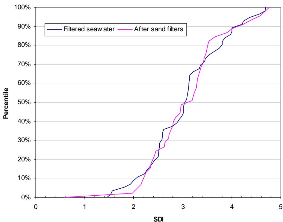
**Figure 9. Frequency distribution plot of silt density index data (after media filters and after cartridge filtration)**
