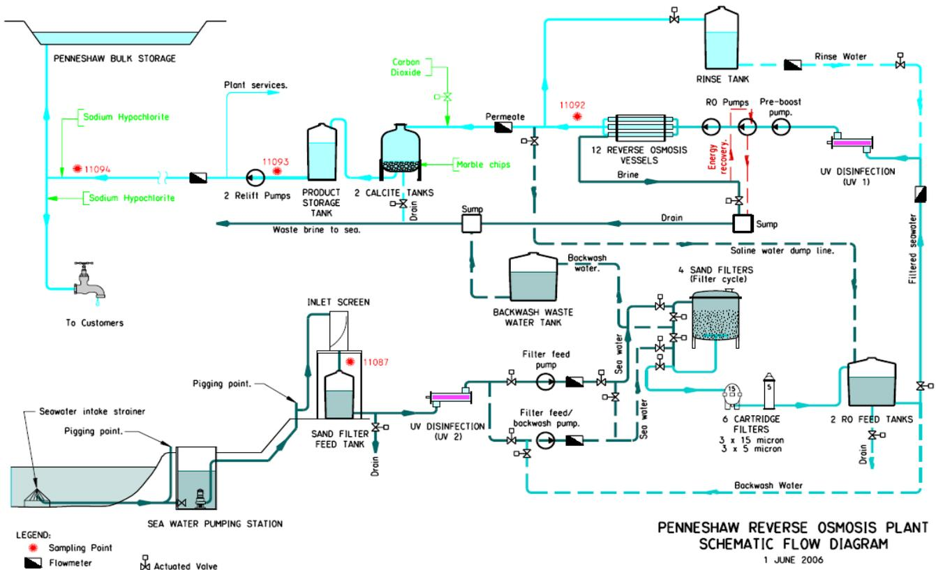
Figure 6. RO plant process flow sheet
