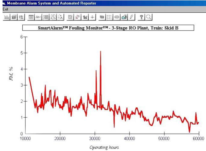
Figure 1.c Non-fouling RO Plant's Fouling Monitor™ History
