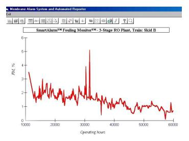
Figure 1.c Non-fouling RO Plant's Fouling Monitor TM History
