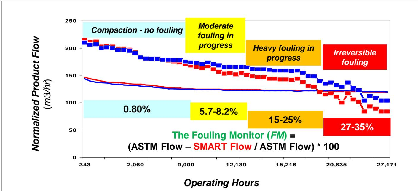
**REAL-TIME MONITORING BY THE SILENT ALARM™ METHOD**
