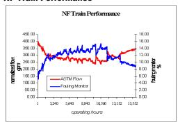
The FM, on the other hand, is based on detecting and quantitatively measuring membrane fouling or scaling as soon as it starts to develop in the system in real-time, eliminating the need for the long-term, ambiguous trending analysis.
