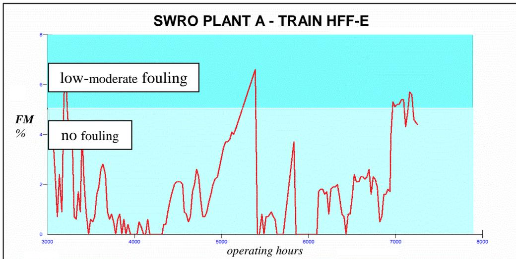
Figure 6 – Real-Time Fouling Monitor of Train HFF-E at Plant A with Non-Fouling HFF Membranes
