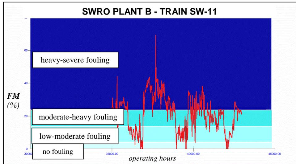
Figure 10 – Real-Time Fouling Monitor of Train SW-11 at Plant B with Fouling HR Membranes
