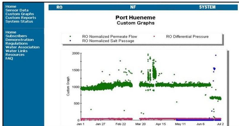
Figure 1 – Standard ASTM-Normalized Flow Profile Monitoring of an RO Plant
