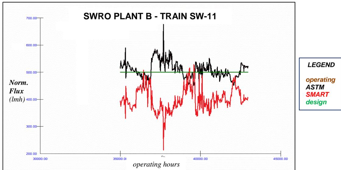
Figure 9 – Real-Time Normalized Flux Decline Profiles of Train SW-11 at Plant B with Fouling HR Membranes
