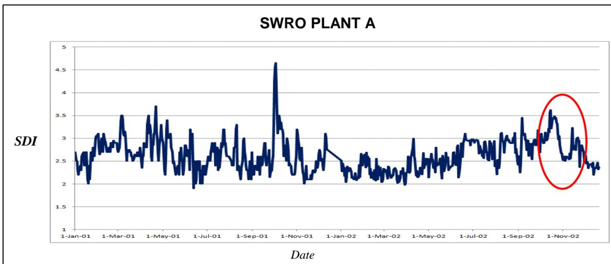
Figure 8 –  $SDI_{15}$  Profile of SWRO Plant A
