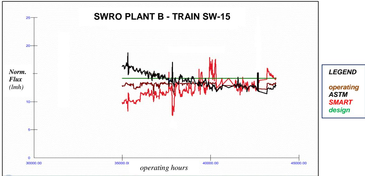
Figure 11 – Real-Time Normalized Flux Declines of Train SW-15 at Plant B with Fouling LF Membranes
