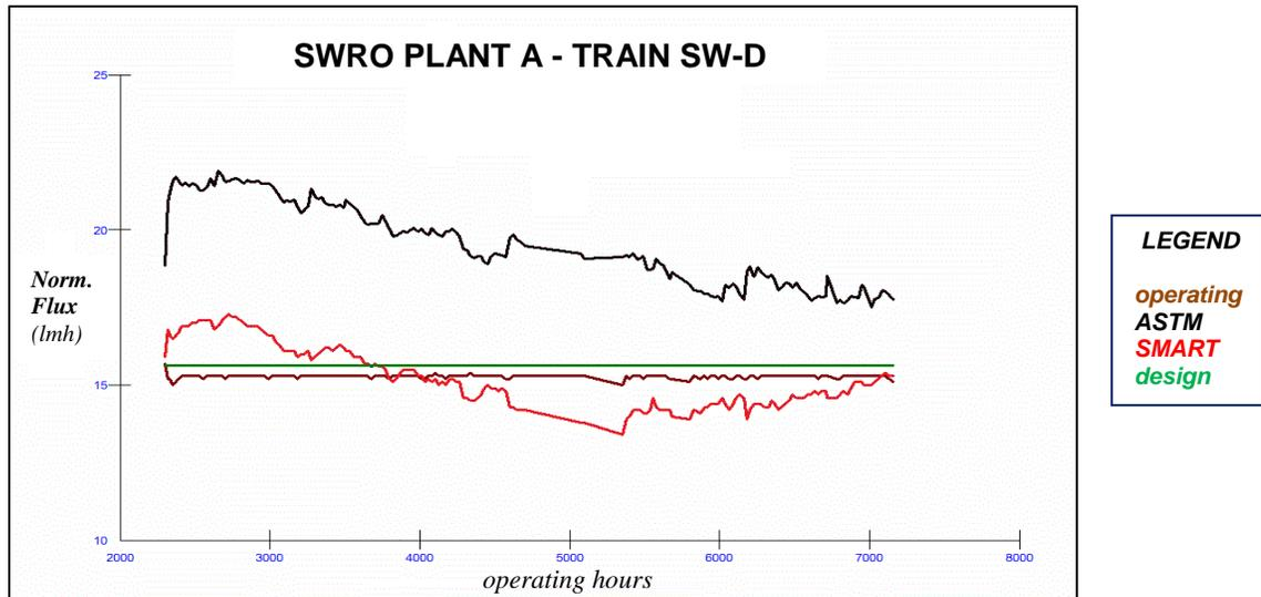
Figure 3 – Real-Time Normalized Flux Decline Profiles of Train SW-D at Plant A with Fouling SW Membranes
