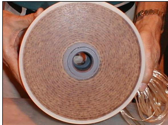
Figure 7.2 Non-fouling HFF membrane
