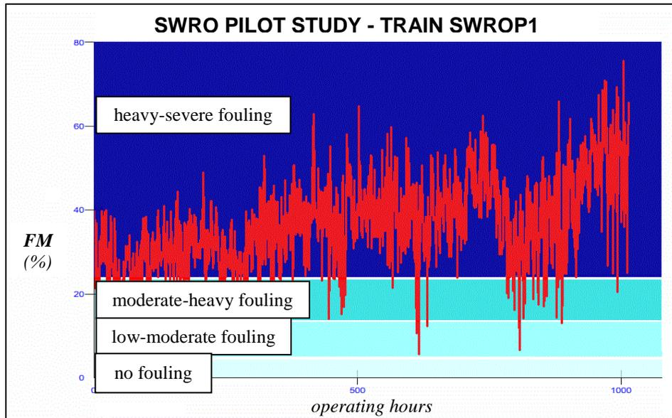
Figure 15 – Real-Time Fouling Monitor of SWRO Pilot Study with Fouling SW Membranes
