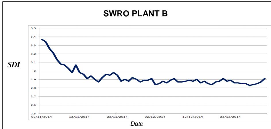
Figure 13 – SDI<sub>15</sub> Profile of SWRO Plant B
