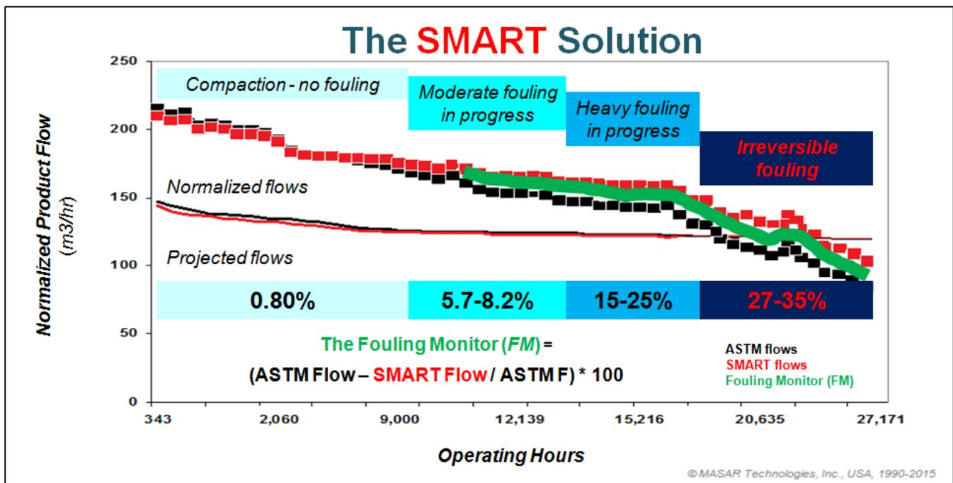
Figure 2 – Real-Time Fouling Monitor of Biofouling High-Brackish RO Plant
