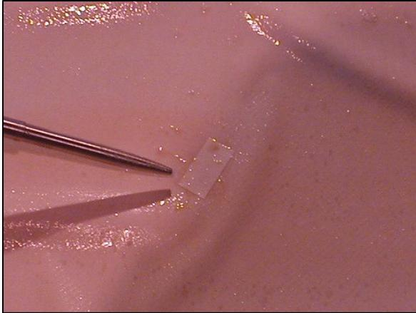
Figure 7.1 Organic fouling on the SW membrane
