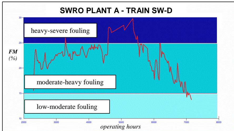
Figure 4 – Real-Time Fouling Monitor of Train SW-D at Plant A with Organically Fouling SW Membranes
