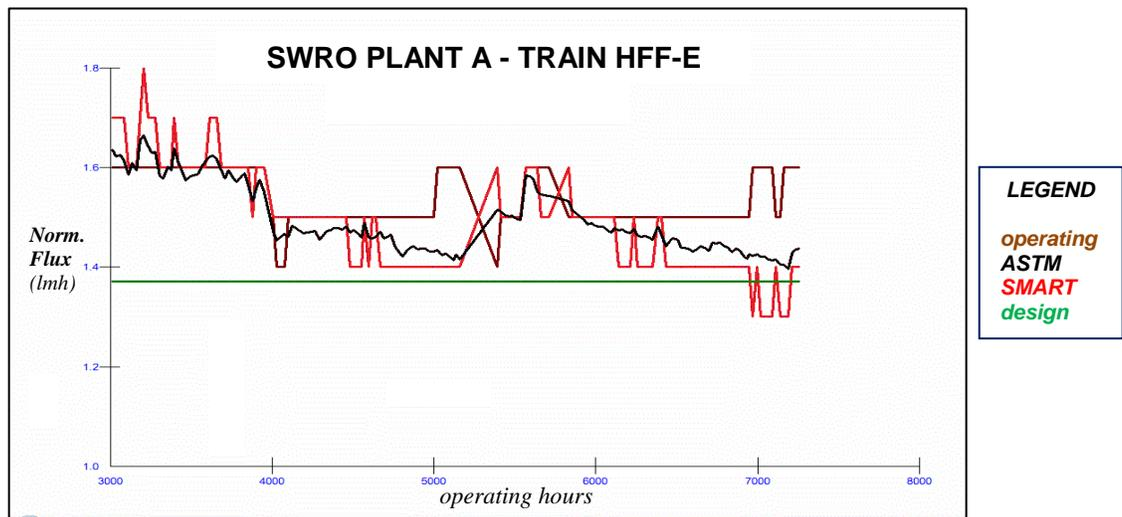
Figure 5 – Real-Time Normalized Flux Decline Profiles of Train HFF-E at Plant A with Non-Fouling HFF Membranes of each other for most of the period, with the corresponding FM averaging 1.77% (Figure 6), indicating non-fouling conditions (Table 2).
