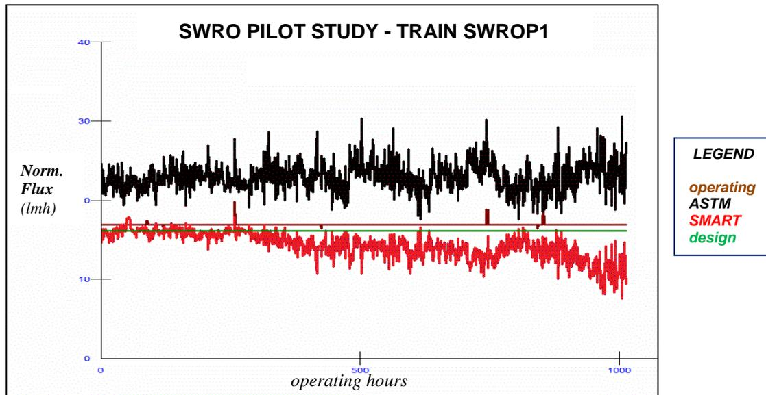
Figure 14 – Real-Time Normalized Flux Decline Profiles of SWRO Pilot Study with Fouling SW Membranes
