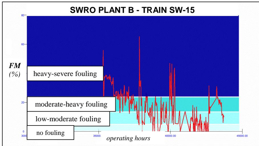
Figure 12 – Real-Time Fouling Monitor of Train SW-15 at Plant B with Fouling LF Membranes
