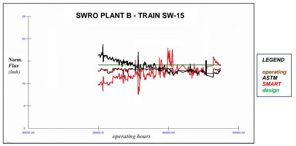
Figure 11 – Real-Time Normalized Flux Declines of Train SW-15 at Plant B with Fouling LF Membranes
