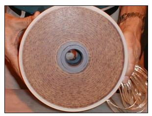
Figure 7.1 Organic fouling on the SW membrane
