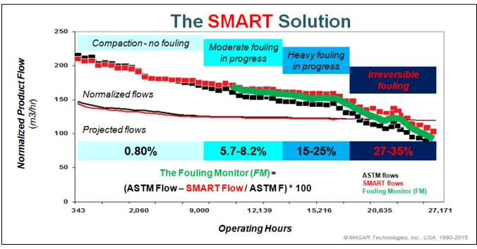
Figure 2 - Real-Time Fouling Monitor of Biofouling High-Brackish RO Plant
