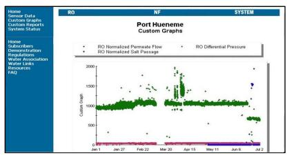
Figure 1 – Standard ASTM-Normalized Flow Profile Monitoring of an RO Plant
