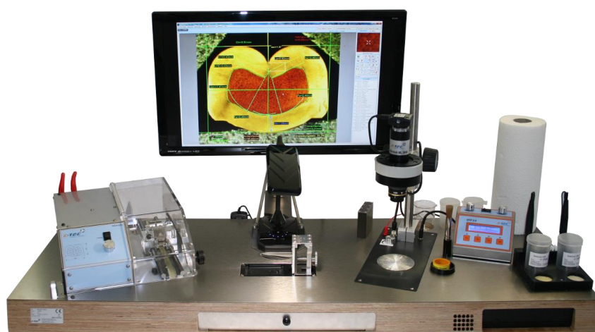
The Microlab ML 3600-pc with integrated mini pc
