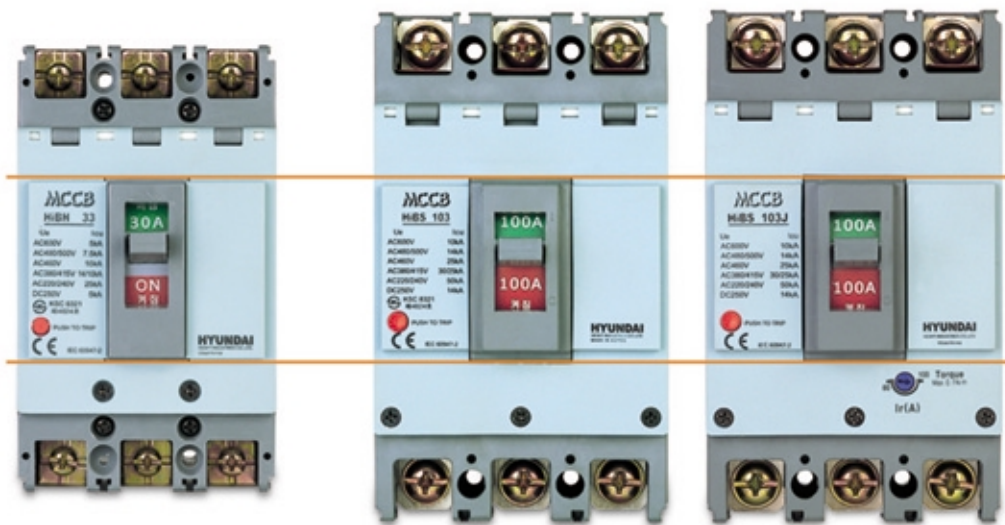
30, 50, 60 & 100AF Non-adjustable In from 3 to 100 A Icu= 5 / 10 kA at 415 V 2, 3, 4 Pole Hydraulic-magnetic Trip Unit
